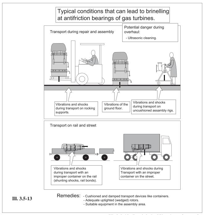
Ill. 3.5-13 (Lit. 3.5-6) Vibrations during the transport with not adequate supported engines or not uptighted r otors can lead to (real) 'brinelling' (example 3.5-1). The experience shows, that such damages can trigger, especially on small high speed engines, even during start up, catastrophic failures in seconds.
